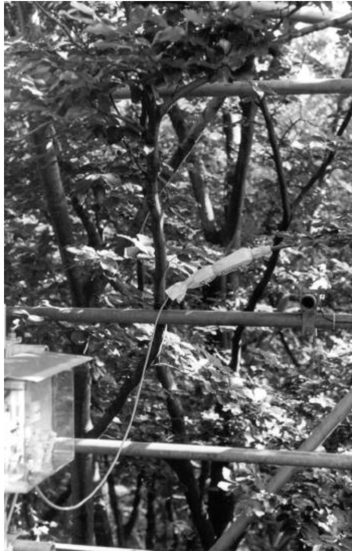
Picture 3.2 Installation of a stem heat balance sensor on a branch in the upper crown level of beech in the forest Aelmoeseneie.
