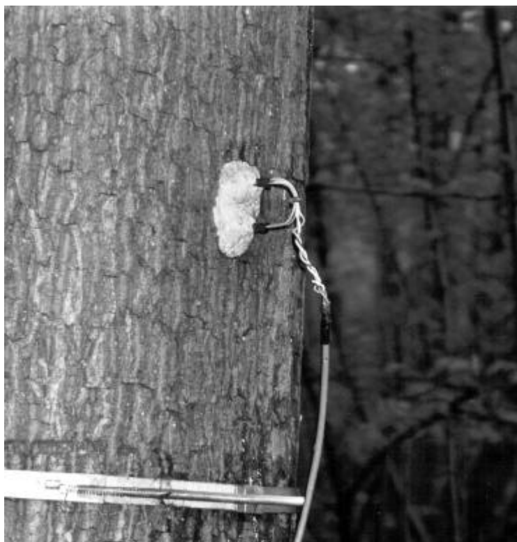
Picture 3.1 Installation of a TDP-sensor in the stem of oak in the forest Aelmoeseneie.
